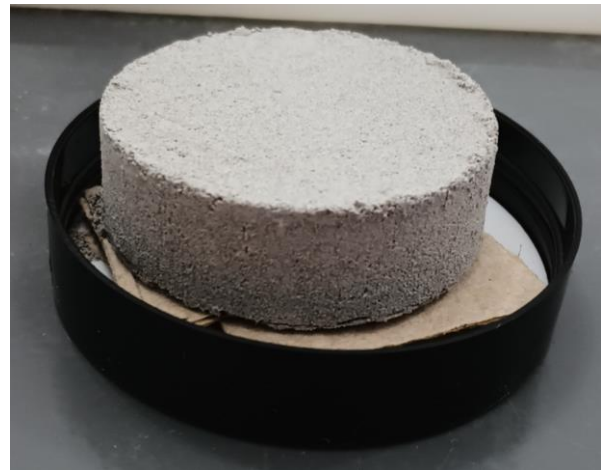
Figure 1: PSS sample shown on the lid of its sample jar, diameter 2 inches.
